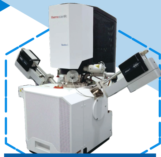
Field Emission Scanning Electron Microscope (FE-SEM-Thermo Scientific) (EDS, Elemental Mapping, SE, BSE, STEM, ESEM, Maps Mineralogy)
