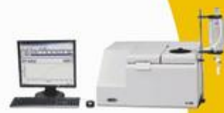
LECO TGA701 (THERMOGRAVIMETRIC ANALYZER)
